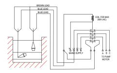
Contact rating: 250V 15A, non-inductive. 250V 10A, inductive. 1.3 HP
