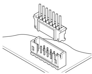
This is a thin, low-profile 2.0mm pitch connector 8.0mm in height after mounting and 4.5mm in width. It is designed to meet the demand for high-density connection of internal wires to printed circuit boards. It is compact, highly reliable and low in cost.
