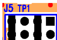
Figure 3: Shows the voltage selection jumpers
