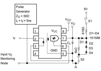
$\ensuremath{\text{C}_{L}}$  is approximately 15pF which includes probe and stray wiring capacitance.
