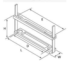
T&B Catalog Number: EAN Number: UPC Number: Description: FCC-3 05414363020479 78621026939 Cable clamp, for flat cables, screw mounting, natural Polyamide 6.6
