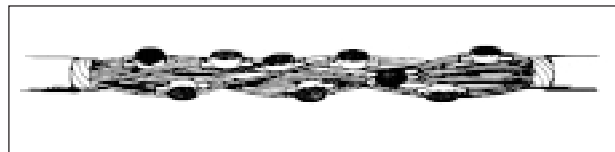
Typical Inline splice made with 3M U1 Scotchlok Connector
