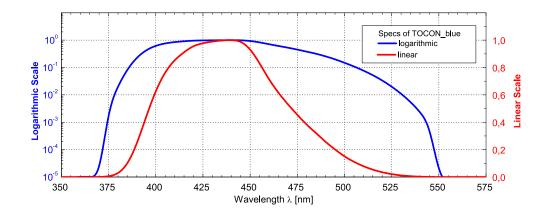
GaP blue light detector with integrated amplifier
