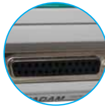
RS-232 25 pin serial interface port
