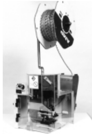
Entry Level Terminator (ELT), 1338600-(x)
