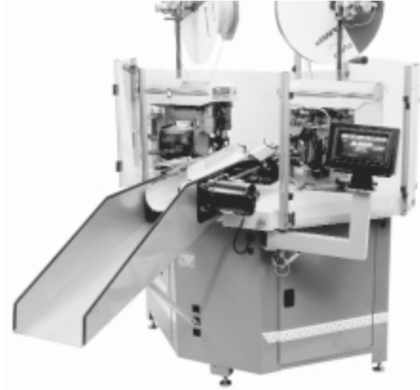
AMPOMATOR CLS IV+ Lead-Making Machines, 356500-1, -2
