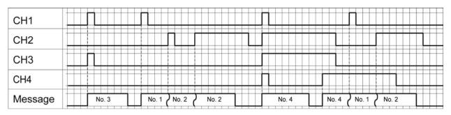
♦ The wavy line in the pulse train indicates a message stopped during playback and the message in conjunction with the input channel is played.
