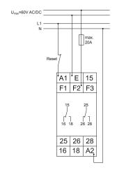
Range 300V, supply voltage 24V AC/DC and fault latch
