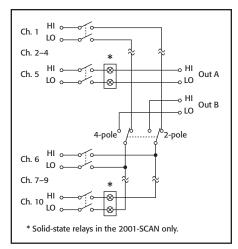
Scanner Configuration for Models 2000-SCAN and 2001-SCAN
