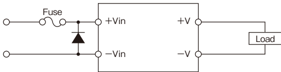
Fig.1-5 Protection for Reversed Input Connection
