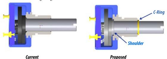
Externally, the design enhancements will be recognized by the C-ring that is visible in front of the bushing. The noted enhancements to this product family will have no effect on form, fit or function. All performance specifications listed on the current data sheet will remain unchanged. These design enhancements allow the potentiometer to withstand higher axial loads typically encountered on installation or removal of mechanical devices from the shaft.
