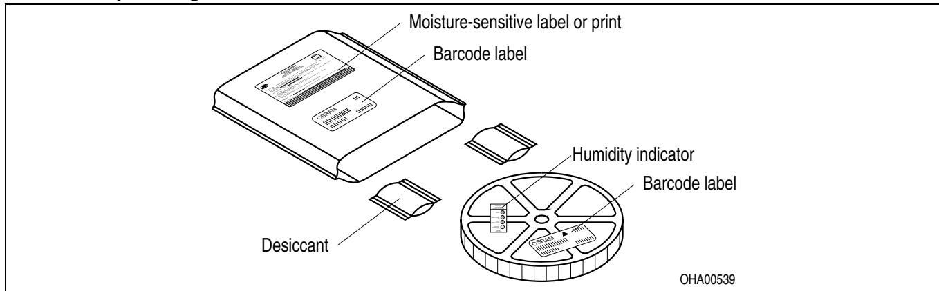
**Note:** Moisture-sensitive products are being packed into a dry bag containing desiccant and a humidity card. Regarding dry packs you will find further information in the internet and in the Short Form Catalog in chapter "Tape and Reel" under the topic "Dry Pack". Here you will also find the normative references like JEDEC.
