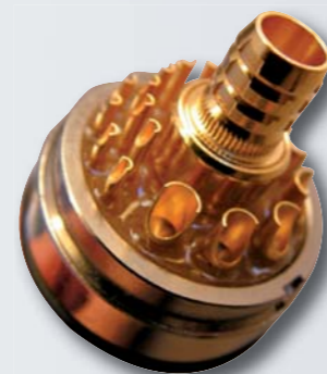
Close-up of the rear of a receptacle, in which potting material was injected.
