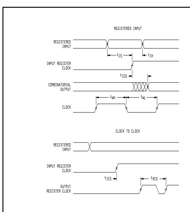
FIGURE 4. Switching waveforms - Continued.
