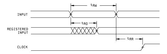
FIGURE 4. Switching waveforms - Continued.
