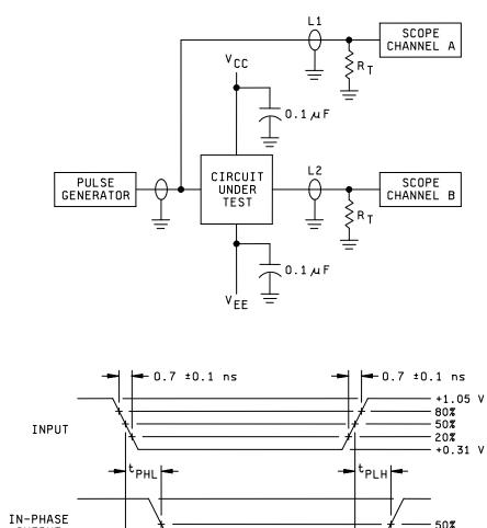
IN-PHASE OUTPUT 50% -⊷|t<sub>PHL</sub> ➡<sup>|t</sup>plh| 80% OUT-OF-PHASE OUTPUT - 50% 20% -<sup>t</sup>thl ⊷<sup>t</sup>⊺LH
