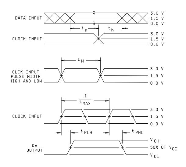
FIGURE 5. Switching waveforms and test circuit.
