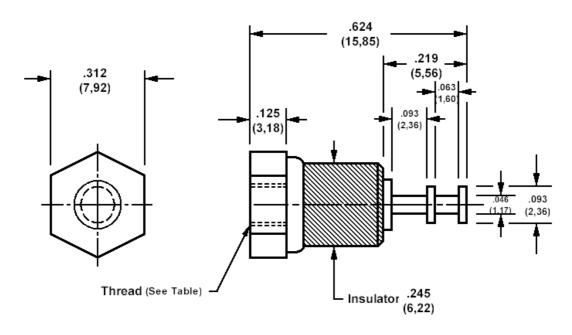
How to order code  $\frac{570\text{-}3648\text{-}\underline{XX}\text{-}\underline{YY}\text{-}\underline{00}}{\text{Basic Part No (XX = thread type, YY = plating finish. See tables for options)}}$
