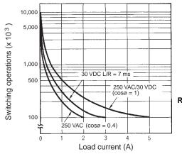
**Reference:** A maximum current of 0.15 A can be switched at 125 VDC ( $\cos\phi = 1$ ) and a maximum current of 0.1 A can be switched at 125 VDC and L/R = 7ms. In both cases, a life of 100,000 operations can be expected. The minimum applicable load is 10 mA at 5 VDC (failure level: P).
