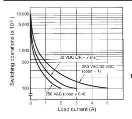
**Reference:** A maximum current of 0.15 A can be switched at 125 VDC ( $\cos\phi = 1$ ) and a maximum current of 0.1 A can be switched at 125 VDC and L/R = 7ms. In both cases, a life of 100,000 operations can be expected. The minimum applicable load is 10 mA at 5 VDC (failure level: P).
