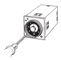
The time required for switching (0.05, 0.1, 0.25, 0.5, 0.75, or 1.0 second) from the star operation to the delta operation of the H3BG-N8/N8H can be selected with the star-delta transfer time selector at the lower right corner of the front panel.
