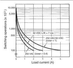
**Reference:** A maximum current of 0.15 A can be switched at 125 VDC ( $cos\phi = 1$ ) and a maximum current of 0.1 A can be switched at 125 VDC and L/R = 7ms. In both cases, a life of 100,000 operations can be expected. The minimum applicable load is 100 mA at 5 VDC (failure level: P).
