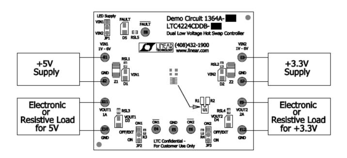
Figure 1. Proper Measurement Equipment Setup
