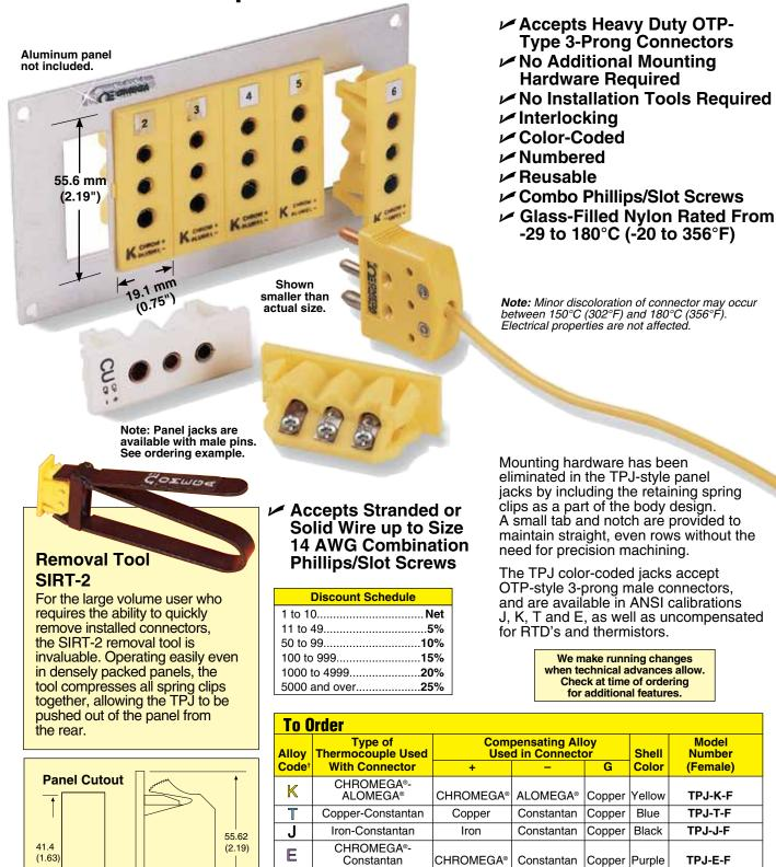
**†** K, T, J and E are ANSI designations. **NOTE**: Type U (Uncompensated) connectors are used with type B thermocouples (Pt/6% Rh-Pt 30% Rh), RTD's and thermistors. To order jacks with male connector prongs, change "**-F**" in model number to "**-M**"; no additional cost.
