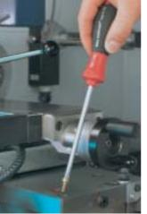
Thanks to Wiha's MagicSpring, inserting and removing TORX® and TORX PLUS® screws is safe and easy.
