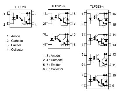
1, 3, 5, 7 : Anode 2, 4, 6, 8 : Cathode 9, 11, 13, 15 : Emitter 10, 12, 14, 16: Collector
