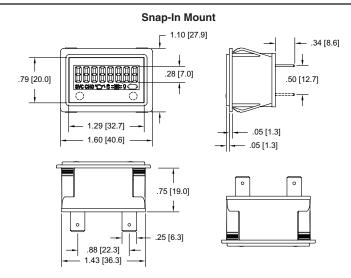
Panel Cutout: 1.45" [36.8mm] x 0.95" [24.1mm] Minimum Panel Thickness: 0.04" [1.0mm] Maximum Panel Thickness: 0.125" [3.18mm]
