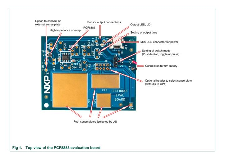
The lower halve is dominated by four sensor areas of different size. The actual circuit is on the upper halve of the board. Arrows indicate the parts of interest which are described more in detail in subsequent sections.
