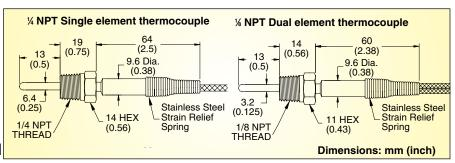
Dual element thermocouple.
