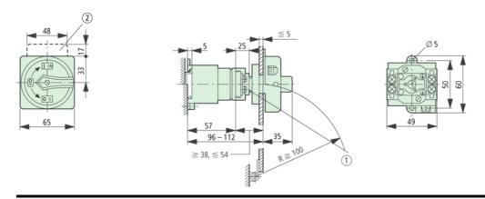
Extension can be extended using ZVV-T0 + ZAV-T0, max. 4 × 25 = 100 mm not included
