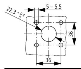
Diameter of drilled hole Door
