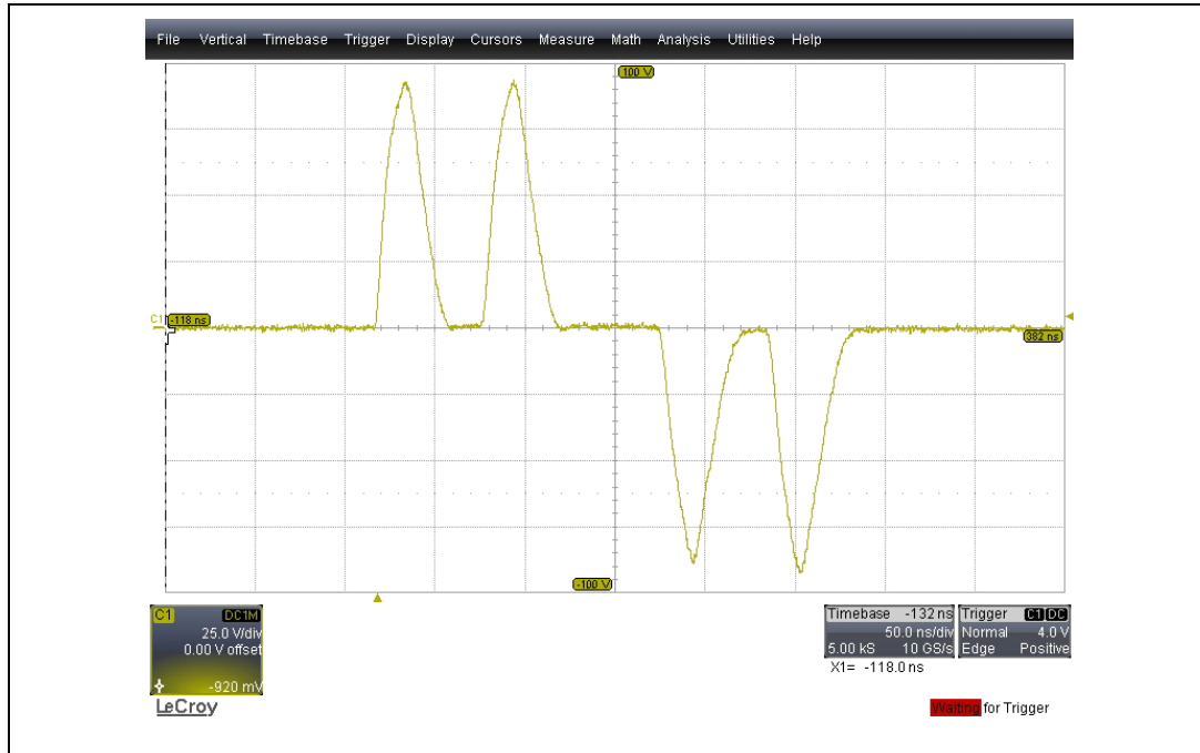
Figure 17. Two positive and two negative “short pulses” with 10 ns time width for inputs IN#, HVP/N/O/1 = ±90 V, load 300 pF // 100 Ω.
