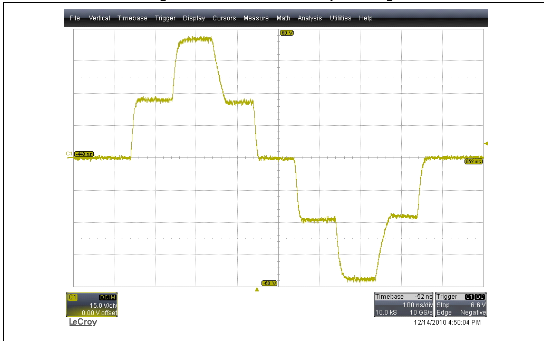
Figure 14. Five-levels HV output voltage
