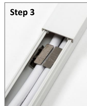
Step 3 Bend over the wings to secure the cables, then fit the lid to the trunking
