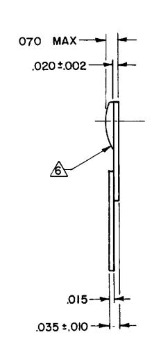
1 TO TEST THE SWITCH AGAINST THE SPECIFIED OPERATING CHARACTERISTICS THE SWITCH MUST BE PLACED IN A HELMHOLTZ COIL FIELD AND GIVEN THE FOLLOWING HISTORY: 35 GAUSS MINIMUM IN DIRECTION "A": 35 GAUSS MINIMUM IN DIRECTION "B" TEST TO THE OPERATING CHARACTERISTICS IN DIRECTION "B" (THIS ASSUMES THE CONVENTION THAT THE DIRECTION OF THE EXTERNAL FLUX OF A MAGNET IS FROM THE NORTH TO THE SOUTH POLE OF A MAGNET)
