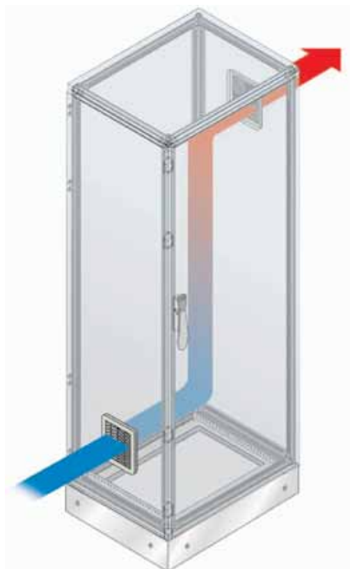
Natural aeration with gratings (IP54 with filter or IP21 without filter).
