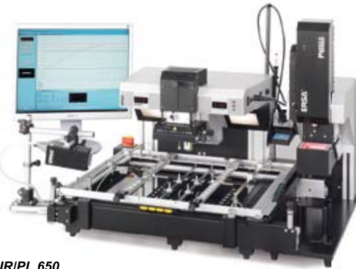
IRIPL 650 DynamicIR heating technology for large (460 mm x 560 mm) PCBs; 4,600 W, 9 zone programmable top & bottom heating zones; precise, easy-to-use motorized Auto "Pick & Place"
