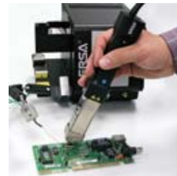
Rapid, simple and safe hand-held component removal
