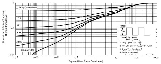
Normalized Thermal Transient Impedance, Junction-to-Ambient
