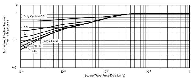
Normalized Thermal Transient Impedance, Junction-to-Case
