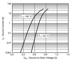
**Source Drain Diode Forward Voltage**
