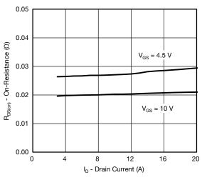
On-Resistance vs. Drain Current
