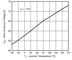
Drain Source Breakdown vs. Junction Temperature
