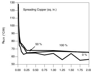
Figure 6. Spreading Copper - Junction-to-Ambient Performance
