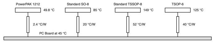
Figure 4. Temperature of Devices on a PC Board
