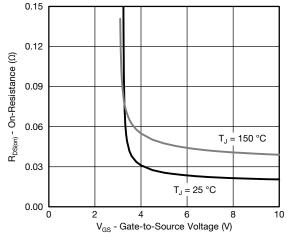
On-Resistance vs. Gate-to-Source Voltage
