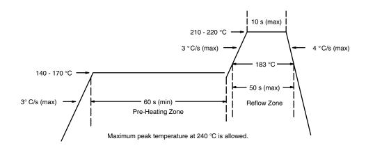
Figure 3. Solder Reflow Temperatures and Time Durations
