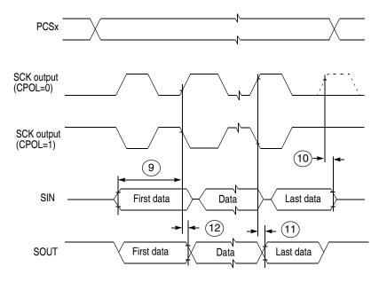
Figure 23. DSPI Modified Transfer Format Timing—Master, CPHA = 1
