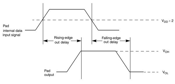
Figure 4. Pad Output Delay
