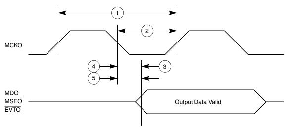
Figure 10. Nexus Output Timing
