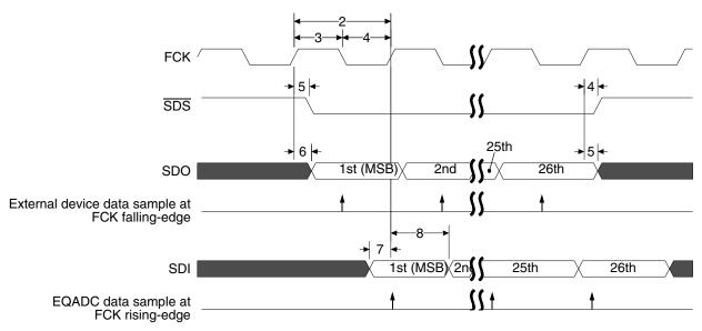
Figure 27. EQADC SSI Timing
