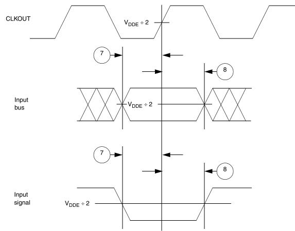
Figure 14. Synchronous Input Timing
