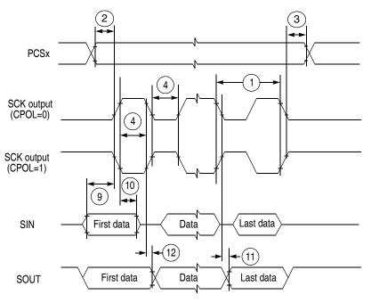
Figure 18. DSPI Classic SPI Timing—Master, CPHA = 0
