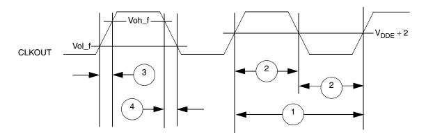
Figure 12. CLKOUT Timing
