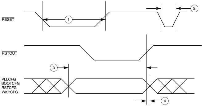
Figure 5. Reset and Configuration Pin Timing
