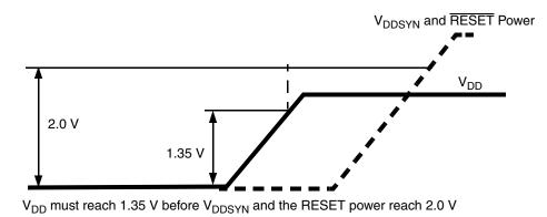
Figure 3. Power-Up Sequence (V<sub>RC33</sub> Grounded)
