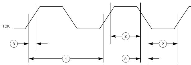
Figure 6. JTAG Test Clock Input Timing
