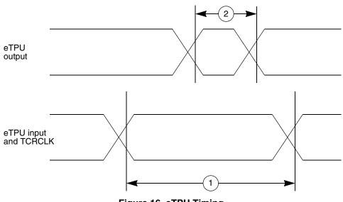
Figure 16. eTPU Timing
