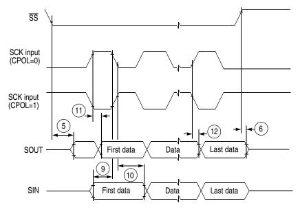
Figure 25. DSPI Modified Transfer Format Timing—Slave, CPHA = 1
