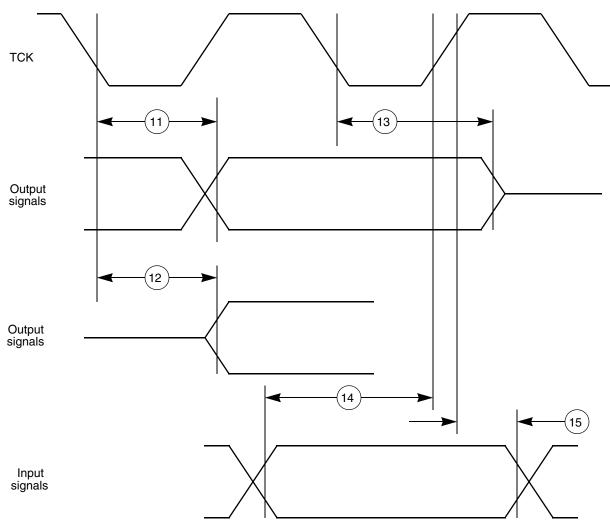
Figure 9. JTAG Boundary Scan Timing
