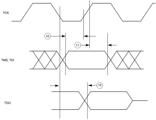
Figure 11. Nexus TDI, TMS, TDO Timing
