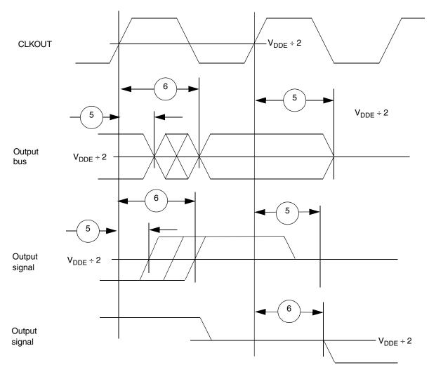
Figure 13. Synchronous Output Timing
