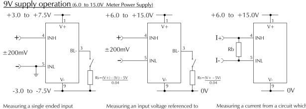
Measuring an input voltage referenced to<br/>a floating supply, i.e. the input voltage<br/>and the meter's power supply are isolated<br/>from each other.Measuring<br/>floating voltage<br/>i.e. the or<br/>supply are isolated<br/>supply are solated<br/>from supply are solated<br/>Ensure solder link LCOM is closed.
