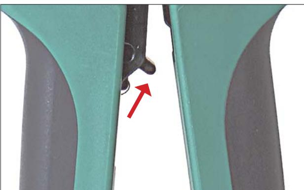
Push the handles slightly together to release the locking lever. Push the release lever of the ratchet upwards. Tool opens automatically.
