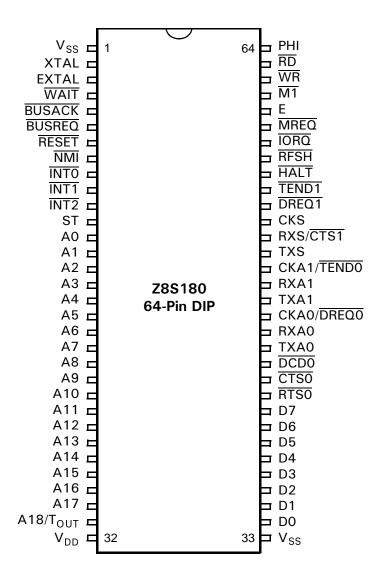
Figure 2. Z8S180 64-Pin DIP Pin Configuration
