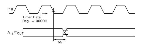
Figure 27. Timer Output Timing
