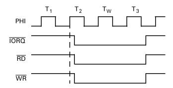
Figure 12. I/O Read and Write Cycles with  $\overline{IOC} = 0$
