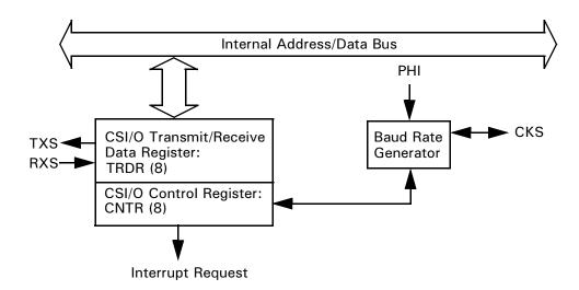
Figure 7. CSI/O Block Diagram
