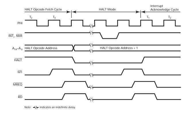
Figure 13. HALT Timing
