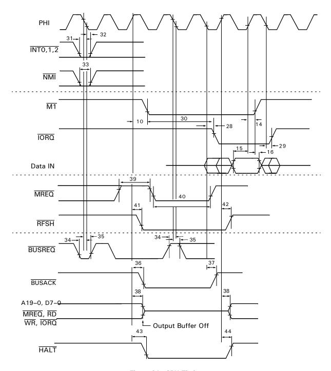
Figure 21. CPU Timing
