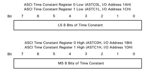
Figure 53. ASCI Time Constant Registers
