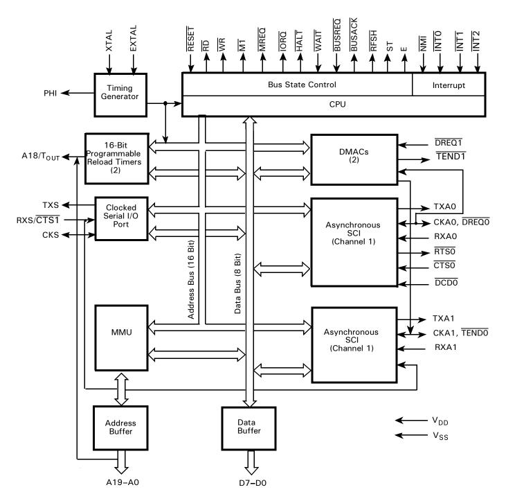
Figure 1. Z8S180/Z8L180 Functional Block Diagram
