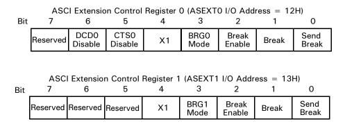
Figure 47. ASCI Extension Control Registers, Channels 0 and 1
