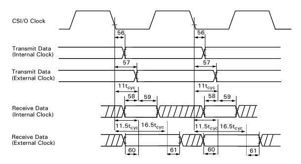
Figure 29. CSI/O Receive/Transmit Timing
