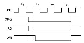
Figure 11. I/O Read and Write Cycles with  $\overline{IOC} = 1$
