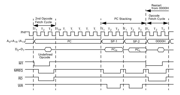
Figure 75. TRAP Timing - 2<sup>nd</sup> Opcode Undefined
