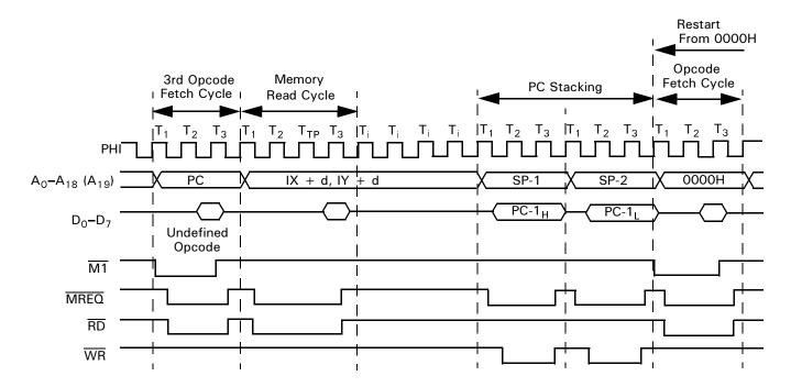
Figure 76. TRAP Timing—3<sup>rd</sup> Opcode Undefined
