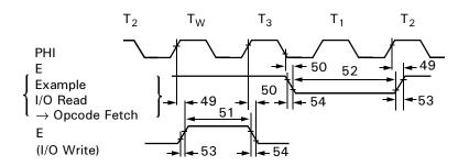
Figure 26. E Clock Timing (Minimum Timing Example of  $\mathbf{P}_{WEL}$  and  $\mathbf{P}_{WEH})$
