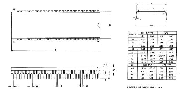
Figure 85. 64-Pin DIP Package Diagram
