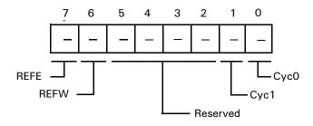
Figure 77. Refresh Control Register (RCR: I/O Address = 36H)
