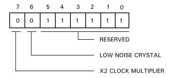
Figure 54. Clock Multiplier Register
