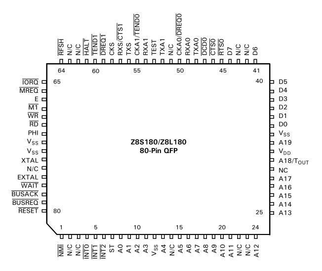
Figure 4. Z8S180/Z8L180 80-Pin QFP Pin Configuration
