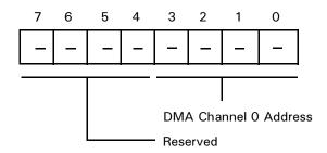
Figure 57. DMA Source Address Register 0B
