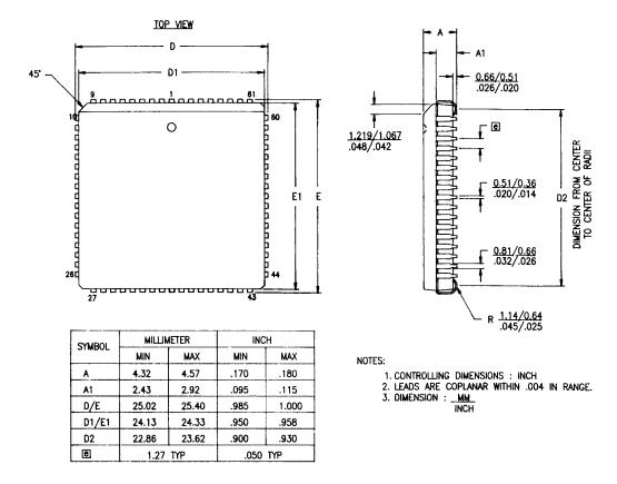
Figure 87. 68-Pin PLCC Package Diagram
