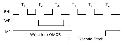
Figure 10. M1 Temporary Enable Timing
