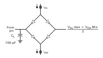
Figure 19. AC Parameter Test Circuit
