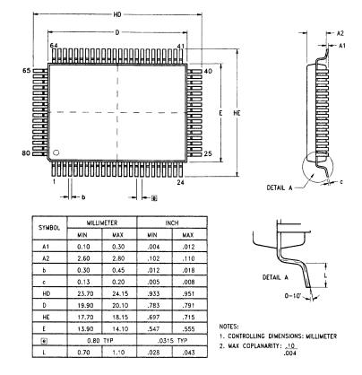
Figure 86. 80-Pin QFP Package Diagram
