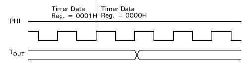
Figure 6. Timer Output Timing
