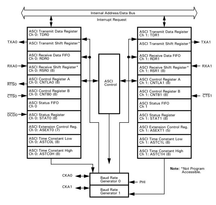
Figure 32. ASCI Block Diagram
