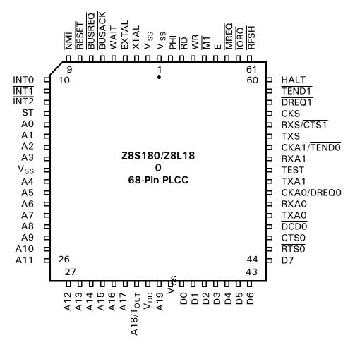
Figure 3. Z8S180/Z8L180 68-Pin PLCC Pin Configuration
