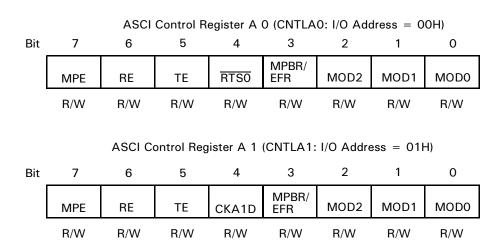
Figure 33. ASCI Channel Control Register A
