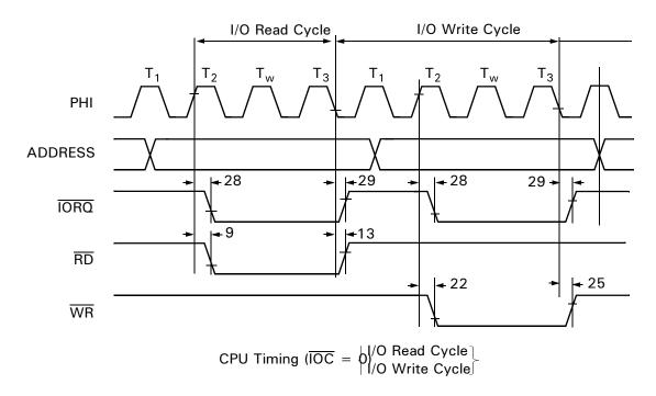
Figure 22. CPU Timing ( $\overline{IOC} = 0$ ) (I/O Read Cycle, I/O Write Cycle)
