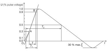
$\begin{array}{ll} \mbox{Front time:} & T_1 = 1.67 \mbox{ x } T = 1.2 \mbox{ } \mu s \ \pm \ 30 \ \% \\ \mbox{Time to half-value:} & T_2 = 50 \mbox{ } \mu s \ \pm \ 20 \ \% \\ \end{array}$
