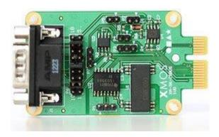
The IS-BUS sliceCARD provides flexible serial connectivity for industrial applications. It includes transceivers for CAN at 1Mbps, LIN at 20Kbps as well as a RS485 at 12Mbps, backed up by associated xSOFTip blocks. All three interfaces may be used simultaneously when connecting via the 0.1" headers. Alternatively one interface can be routed to the DB9 connector
