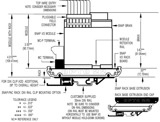
HORIZONTALLY TO USE SNAP I/O WITHOUT MODULE HOLD-DOWN SCREWS)
