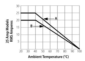
A: Single relay or with 0.75" spacing between relays. Derate above 40 °C; subtract 0.5 amp/°C.
