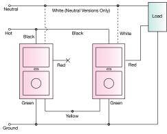
Note: \* Load can not exceed the rating of one switch.
