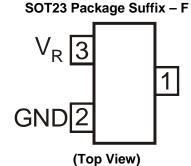
Pin 1 floating or connected to pin 2
