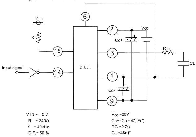
(\*) Please mount the capacitor for the voltage amends as much as possible near hybrid IC.
