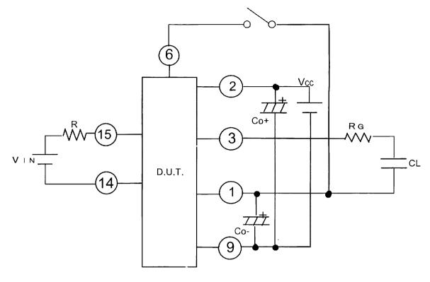
V | N = 5 VR = 340 $\Omega$   $V_{CC}$  = 20V RG = 2.7 $\Omega$ CL = 48nF Co+=Co-=47 $\mu$  F
