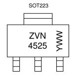
ZVN 4525 = Product Type Marking Code YWW = Date Code Marking Y or  $\overline{Y}$  = Last Digit of Year (ex: 5= 2015) WW or  $\overline{W}W$  = Week Code (01~53)
