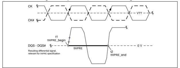
Figure 41 – Method for calculating tWPRE transitions and endpoints
