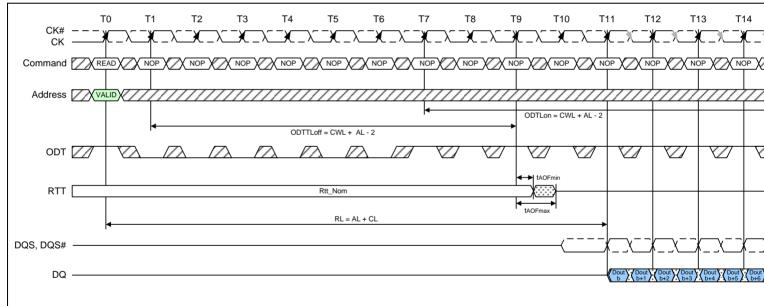
Figure 76 – ODT must be disabled externally during Reads by driving ODT low. (CL = 6; AL = CL - 1 = 5; RL = AL + CL = 11; CWL = 5; ODTLon = CWL + AL - 2 = 8; ODTLoff = CWL + AL
