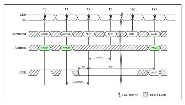
Figure 66 – Active Command to Power-Down Entry
