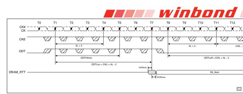
Figure 74 – Synchronous ODT Timing (AL = 3; CWL = 5; ODTLon = AL + CWL - 2 = 6; ODTLoff = AL + CW
