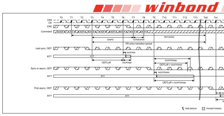
Figure 84 – Synchronous to asynchronous transition after Refresh command (AL = 0; CWL = 5; tANPD = V
