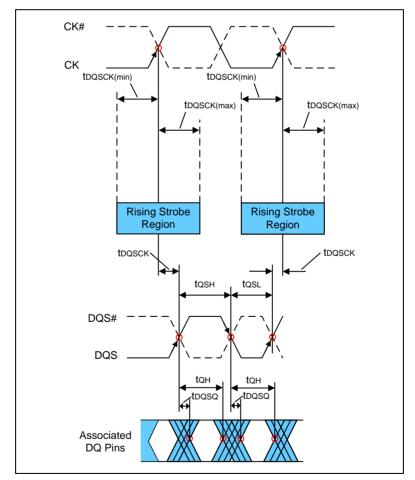
Figure 23 – READ Timing Definition
