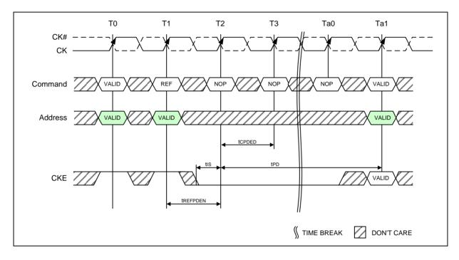
Figure 65 – Refresh Command to Power-Down Entry
