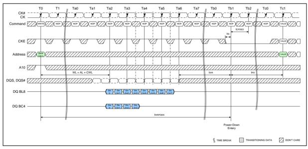
Figure 62 – Power-Down Entry after Write
