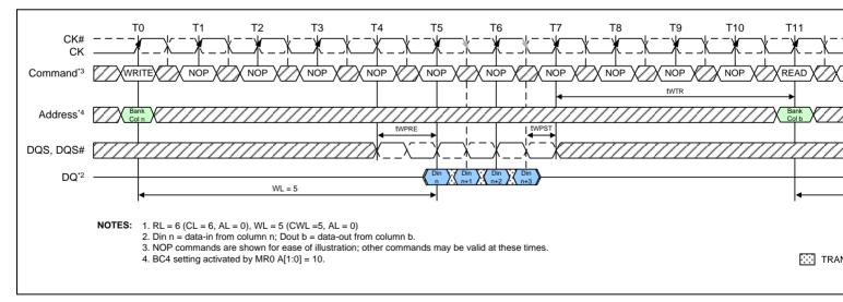
Figure 52 – WRITE (BC4) to READ (BC4)
