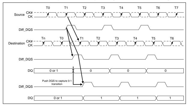
Figure 13 – Write Leveling Concept
