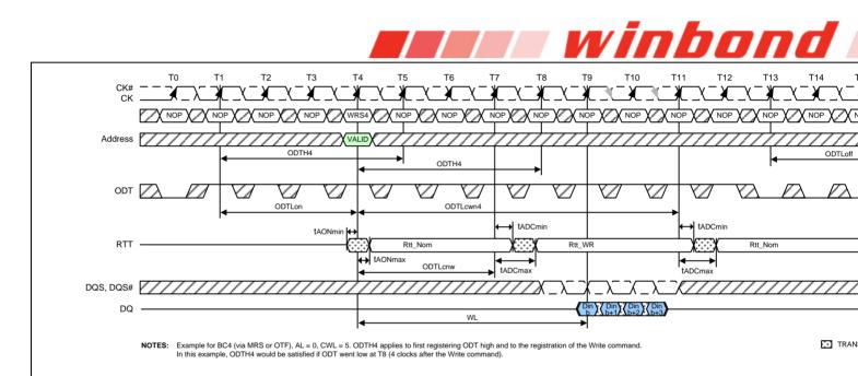
Figure 77 – Dynamic ODT: Behavior with ODT being asserted before and after the write
