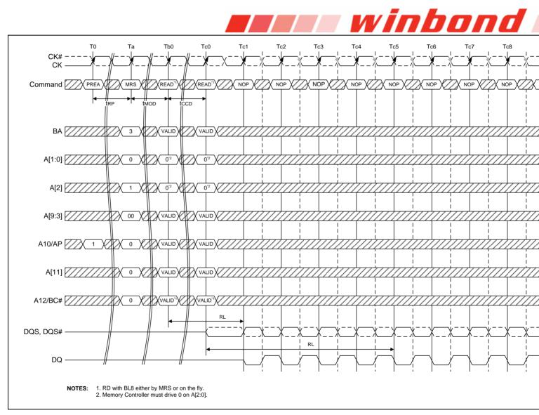
Figure 18 – MPR Readout of pre-defined pattern, BL8 fixed burst order, back-to-back readout
