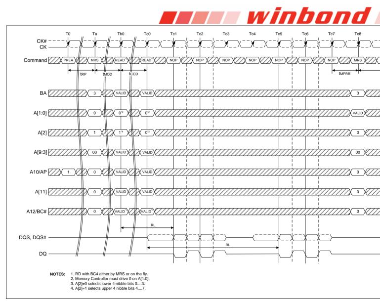
Figure 20 – MPR Readout of pre-defined pattern, BC4, upper nibble then lower nibble
