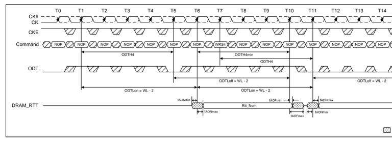
Figure 75 – Synchronous ODT (BL = 4, WL = 7)
