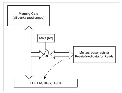
Figure 16 – MPR Block Diagram
