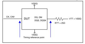
Figure 98 – ODT Timing Reference Load
