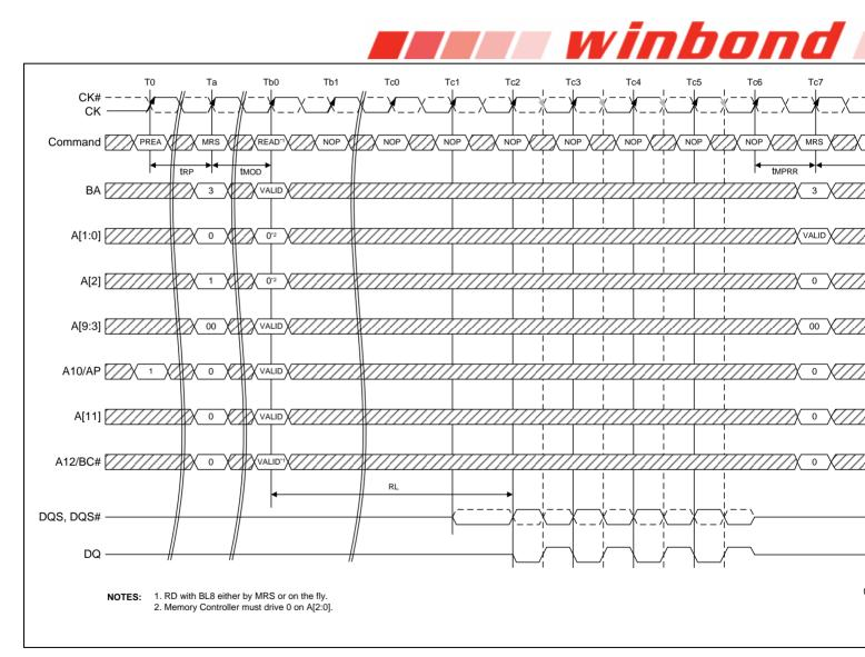
Figure 17 – MPR Readout of pre-defined pattern, BL8 fixed burst order, single readout
