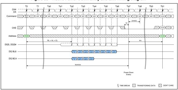
Figure 59 – Active Power-Down Entry and Exit Timing Diagram
