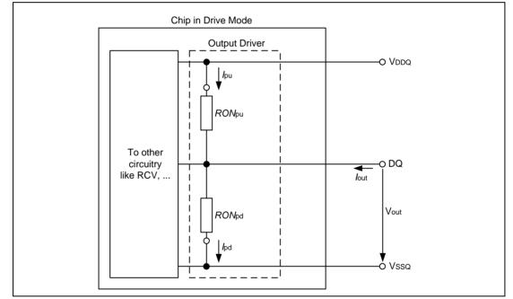
Figure 96 – Output Driver: Definition of Voltages and Currents
