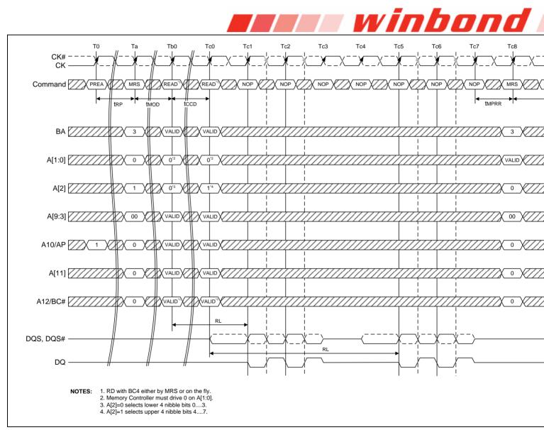
Figure 19 – MPR Readout pre-defined pattern, BC4, lower nibble then upper nibble
