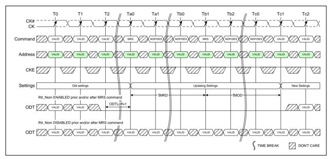
Figure 3 – tMRD Timing
