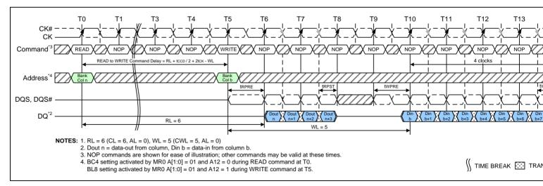
Figure 36 – READ (BC4) to WRITE (BL8) OTF
