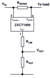
ZXCT1009 with additional current limiting Resistor R<sub>LIM</sub>.
