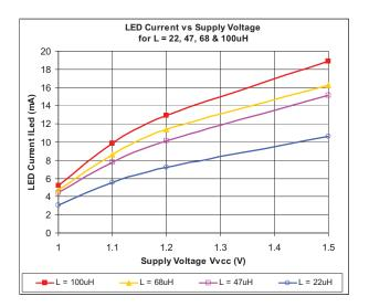
Figure 3 The LED current vs the supply voltage for various inductor values
